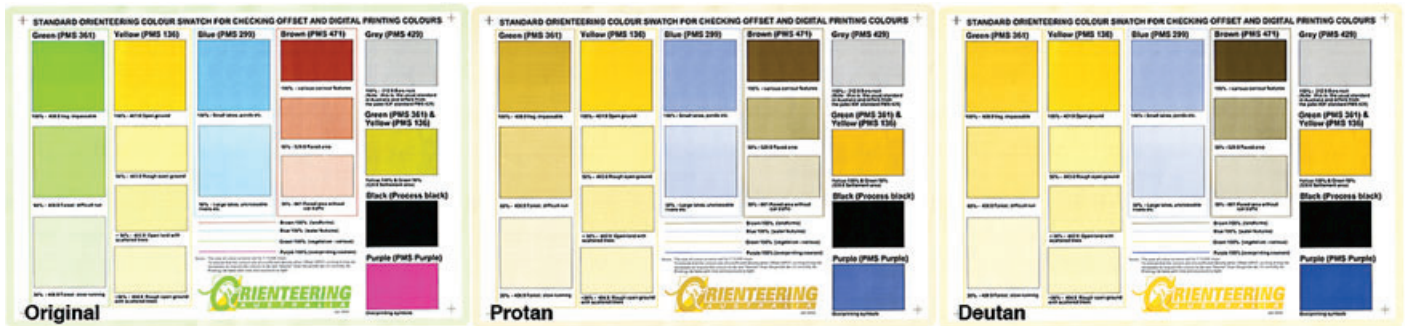
Figure 3. The PMS colour swatch issued by Orienteering Australia for checking offset and digital printing of orienteering maps plus simulations of views by colour defective orienteers rendered using Vischeck plug-ins for Adobe Photoshop (www.vischeck.com). Left: The original colour scheme. Middle: Portrayed as viewed by an orienteer with a protan defect. Right: Portrayed as viewed by an orienteer with a deutan defect.
